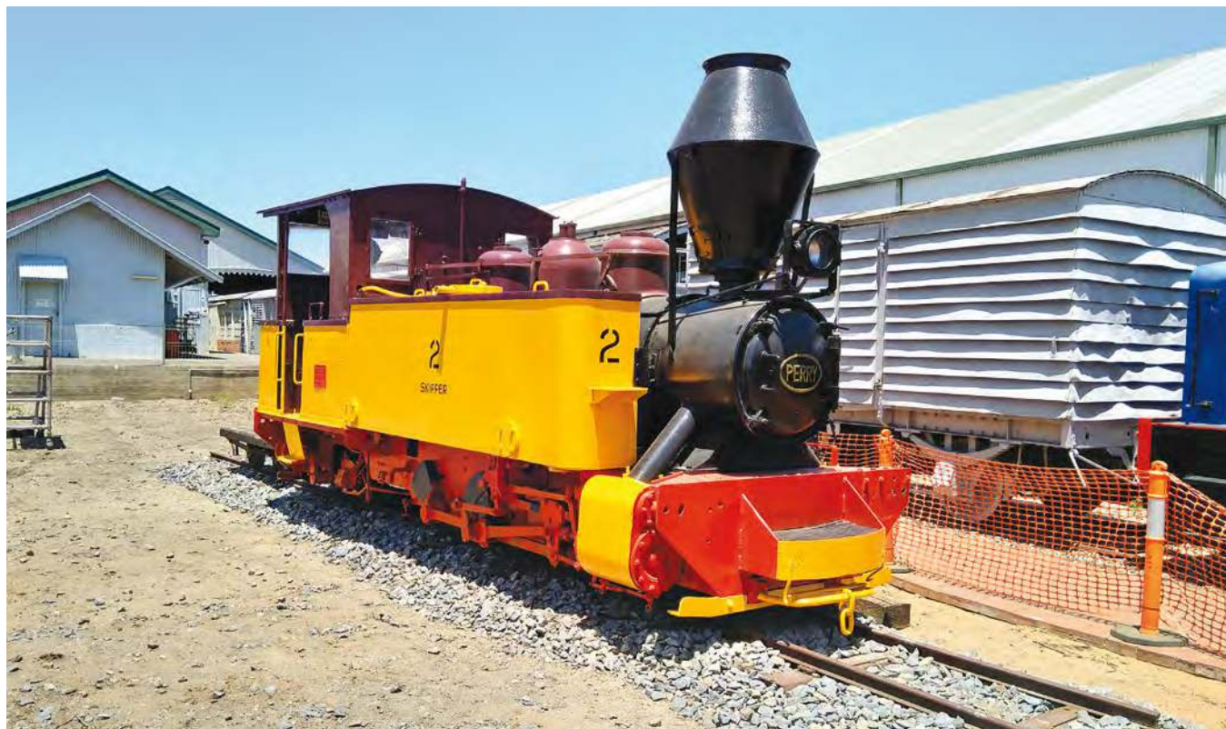
Above: Built in 1946, Skipper was one of 19 2ft (610mm) gauge 0-6-2T and 0-4-2T locomotives built by Perry Engineering at Mile End, near Adelaide, between 1934 and 1952 for various Queensland sugar mills. Skipper was originally owned by Millaquin Mill in Bundaberg, and was later transferred to nearby Qunaba Mill where it remained in loyal service until its withdrawal in 1980. In 1981 Skipper returned home to South Australia and was displayed at the ARHS Mile End Railway Museum until 1986 when it was transferred to the Port Dock Station Museum (now the National Railway Museum) at Port Adelaide, and is seen there on Friday 11 January. It has become a most popular exhibit, especially with children. A museum volunteer said: “ Skipper always brings so much joy to the children...” Effie Kelly Below: Ex-QR PB 15 4-6-0 No.448, recently returned to Queensland Pioneer Steam Railway operations, is seen doing the second run from Bundamba to Swanbank on Sunday morning 10 February. It appears the fireman is leaning out of the cab to ensure the flashing lights at the nearby level crossing – about 100m in front of the engine – are fully operational. Mike Martin
