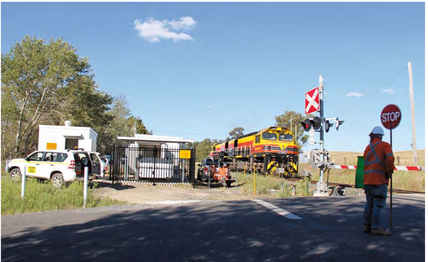
On Sunday, 17 February, a test ‘train’ comprising Southern Shorthaul Railroad BRM Class units 001 and 002 was used to test signalling at the new Georges Plains crossing loop and the ‘follow on’ block post at Wimbleton. The two locomotives are seen at the Bathampton Road level crossing at Wimbleton on a test run as technicians check the track circuits in the equipment hut to the left. John Hoyle
