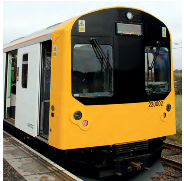
The converted London Underground D78 stock unit manoeuvres around the yard at Bo'ness on October 12, 2018. (Paul Gerrard)
