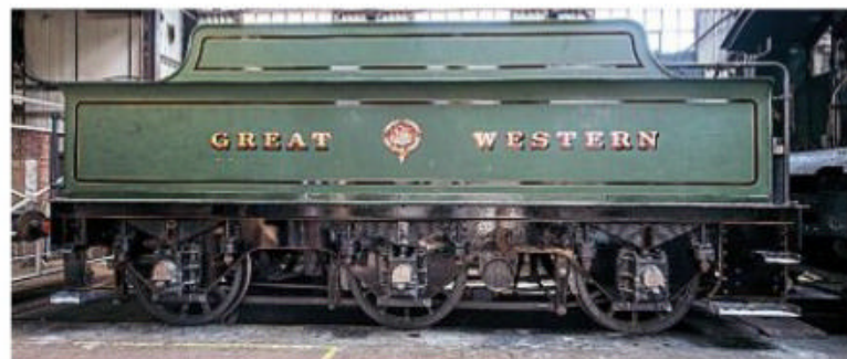
The Churchward 3,500-gallon tender of No. 2999 following lettering and application of the garter crest at Didcot. The crest has been placed according to the practice of the period so it lined up with the centre axlebox. Note how the paintwork has been flattened down before varnishing. FRANK DUMBLETON
