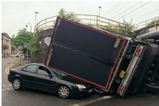
Vehicles colliding with railway bridges is a daily occurrence. Some bridges have a protective or sacrificial beam, which means services can be cautioned, minimising delays, while others need a visual inspection. In this incident at Stoke-on-Trent on August 25, 2016, the errant HGV driver tried to get under a 13ft 3in bridge at Stoke Road/Station Road junction, and while the beams did their jobs, the HGV wrote off a Ford Mondeo. NETWORK RAIL
