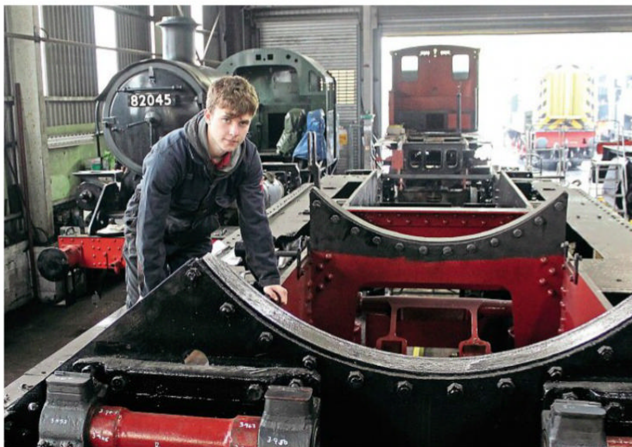
Jacob undertakes work on the frames of GWR 'Hall' 4-6-0 No. 4930 Hagley Hall in the Bridgnorth workshops.
