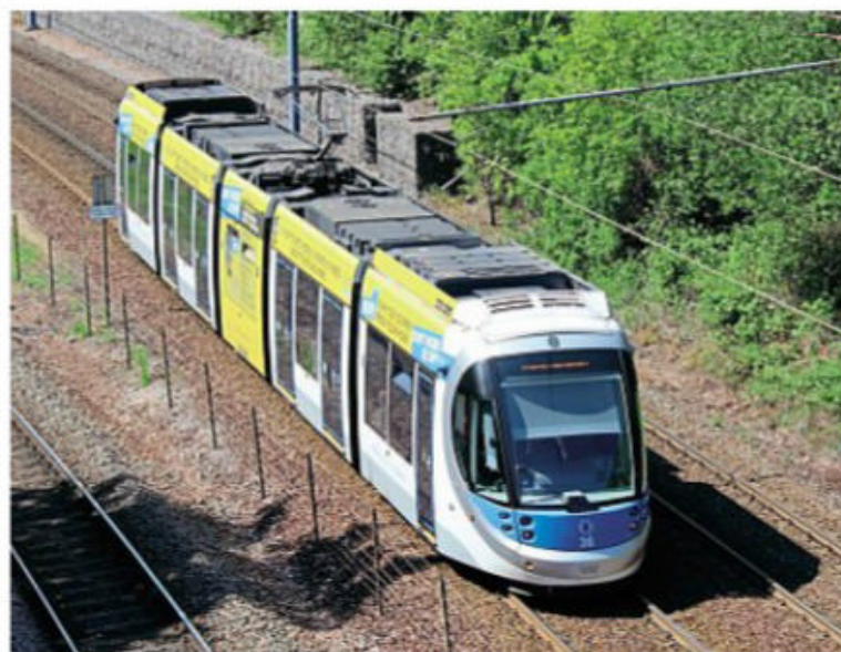
ROOF-TOP BATTERIES: This elevated view of West Midlands Metro tram No. 36, as it departs The Hawthorns for Wolverhampton St Georges on May 14, shows the battery packs that are being fitted to the fleet above both cab ends. Around half the fleet of 21 trams has had the batteries fitted so far, but all will need to be so equipped before services can begin over the wire-free extension from New Street station to Centenary Square later this year. MIKE HADDON
