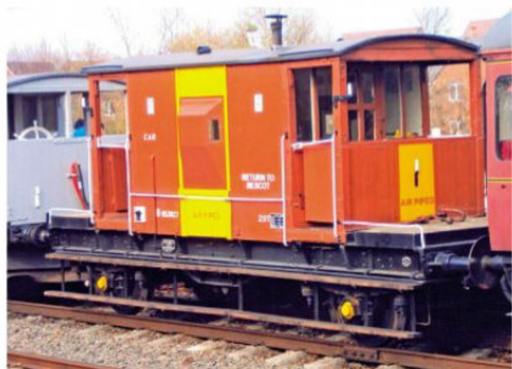
TOPS-coded CAR brakevan is air-piped and part of the Chasewater Railway fleet. S F LAPPAGE
