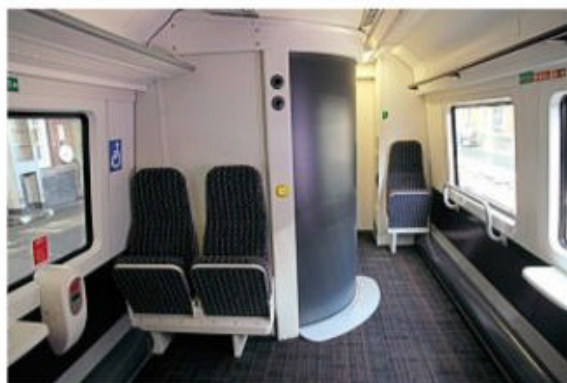
The interior of the refurbished Class 172 showing the 2+2 seating and the accessible toilet and tip-up seat area.
