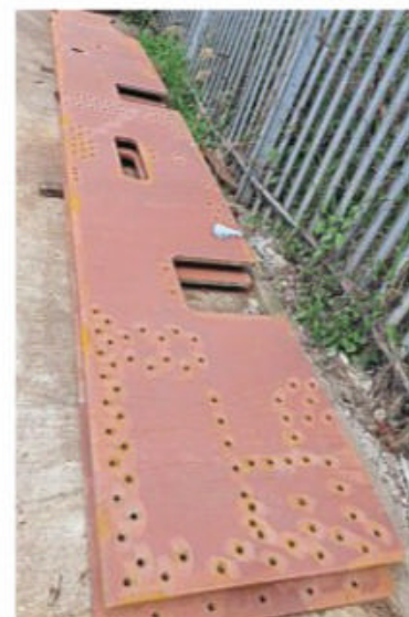
The frame plates for No. 3840 County of Montgomery after drilling at Goodman Metal Works in Nottingham prior to delivery to Tyseley. RICHARD GOODMAN
