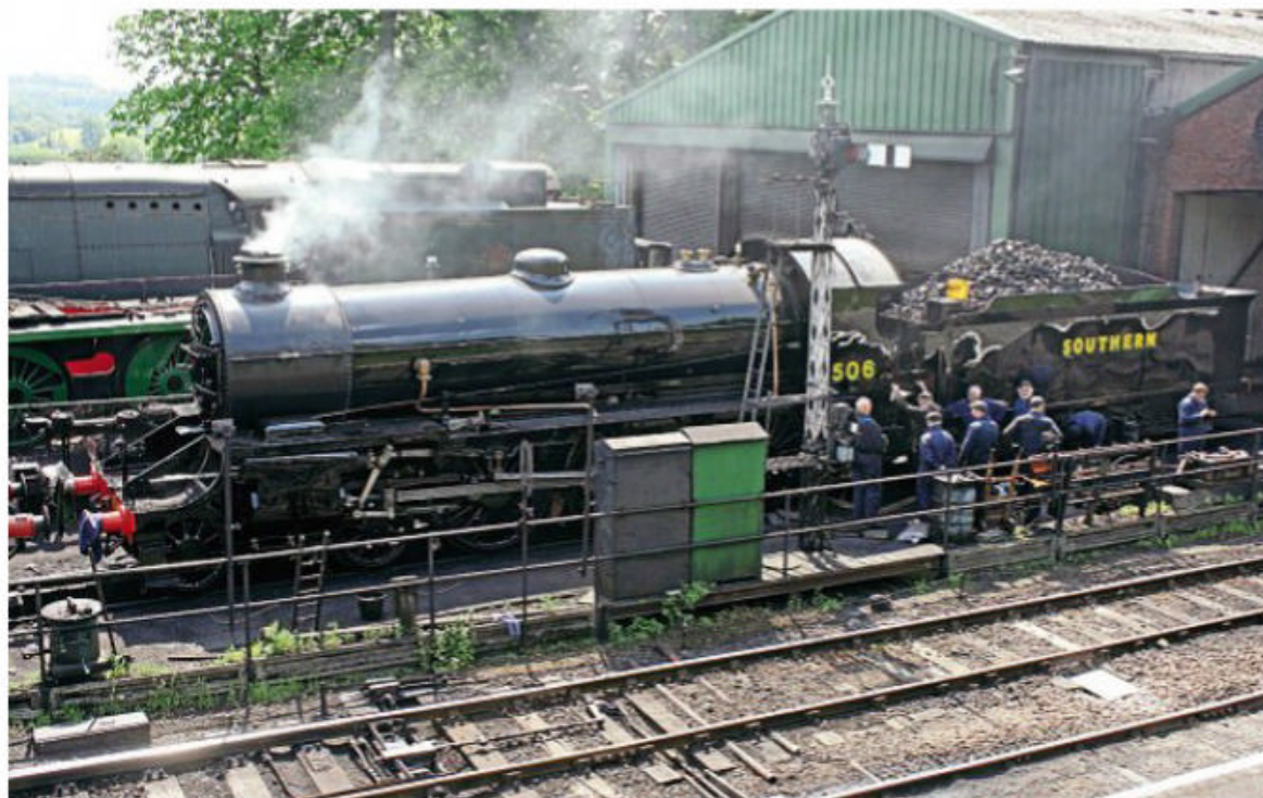
The Churchward 3,500-gallon tender of No. 2999 following lettering and application of the garter crest at Didcot. The crest has been placed according to the practice of the period so it lined up with the centre axlebox. Note how the paintwork has been flattened down before varnishing. FRANK DUMBLETON
