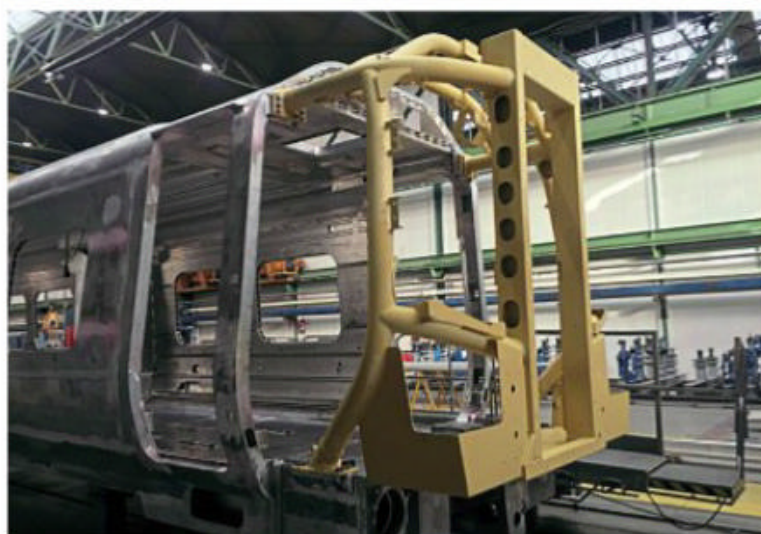
The bodysell of a Class 196 under construction at CAF's Beasain factory, Spain.
